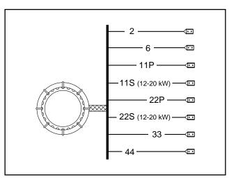
Figure 4. Stator Assembly Leads
